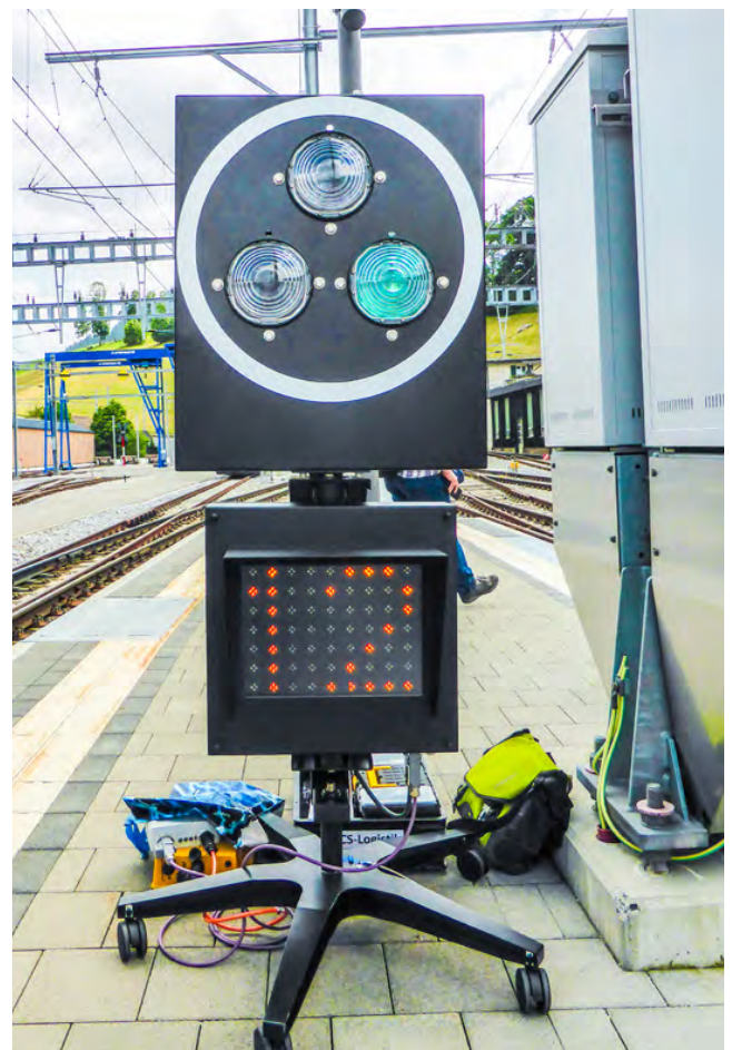
The LED signal and LED route indicator. Photo Daniel Pixley.
