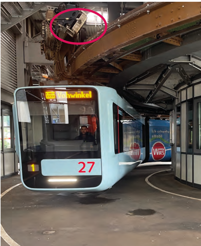
Top, IRSE Swiss Section travellers in front of the Schwebebahn. Left, a train at the depot Oberbarmen making the turning loop. In front of the wheel diagonally is the balise reader (circled). Above, a train arriving into Werther Brücke.
