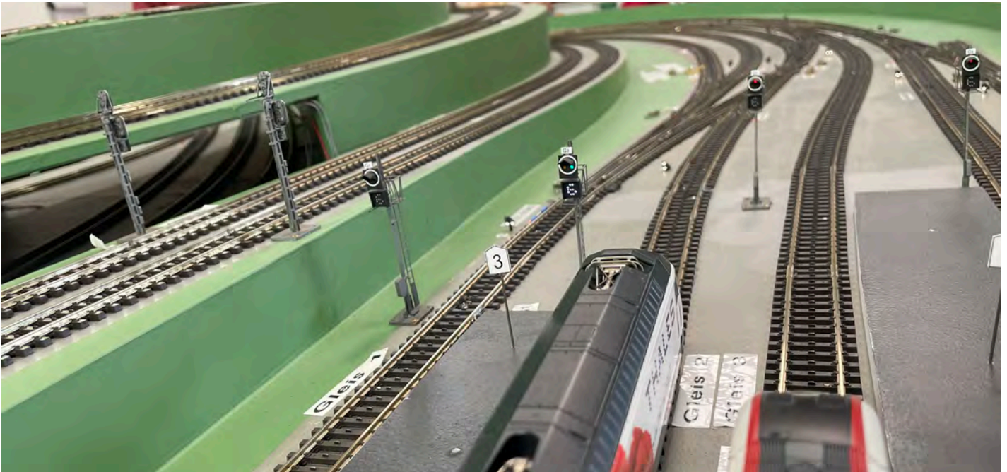
Above: Train in track 2 about to depart, signal G2 shows 'proceed 6', which means 60km/h. Also, visible multiple dwarf signals, one showing a clear aspect, others stop. Right: Nadia Hürlimann explaining the operation of electromechanical interlocking station Zetthausen. Bottom right: Beatrice Müller and Markus Montigel shortly before he was made an Honorary Fellow.
